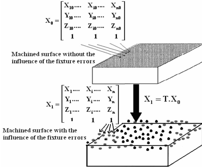
Figure 3: Tensorial modelling of the influence of the fixture errors.
