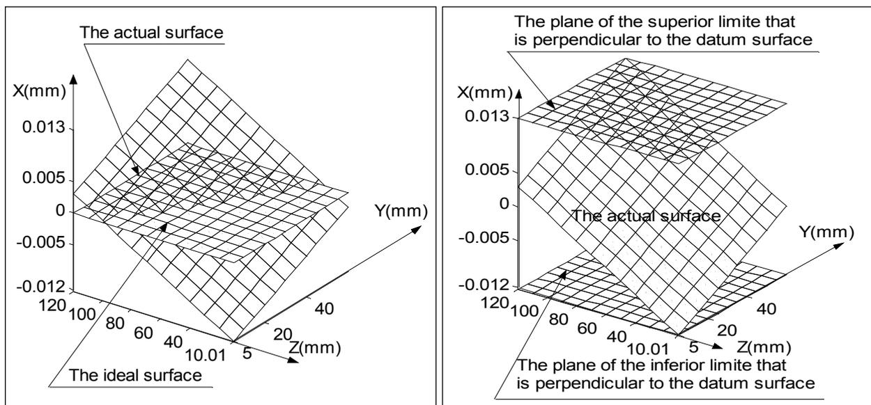
Figure 10: Geometric defaults that influence the perpendicularity of the machined surface 8 by report the datum surface 9 while using the 2<sup>th</sup> fixture location
