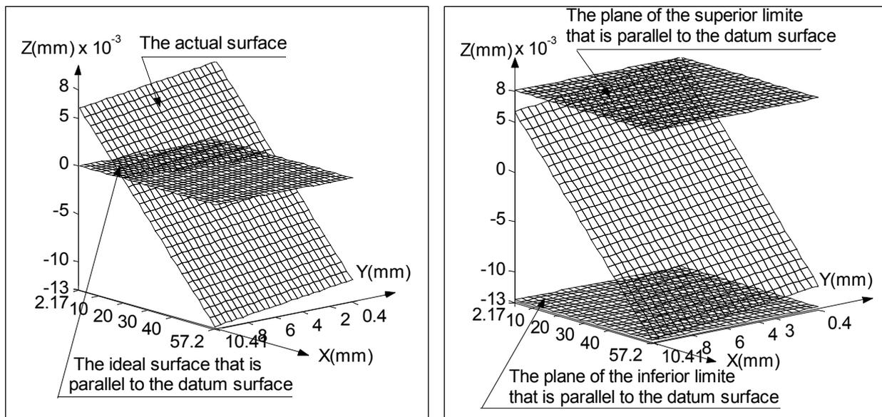
Figure 7: Geometric defaults that influence the parallelism of the machined surface 1 by report the datum surface 6 while using the 1<sup>st</sup> fixture location.
