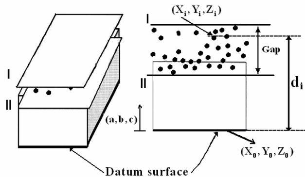
Figure 4: Interpretation of geometric defaults that influences the respect of the condition of parallelism.
