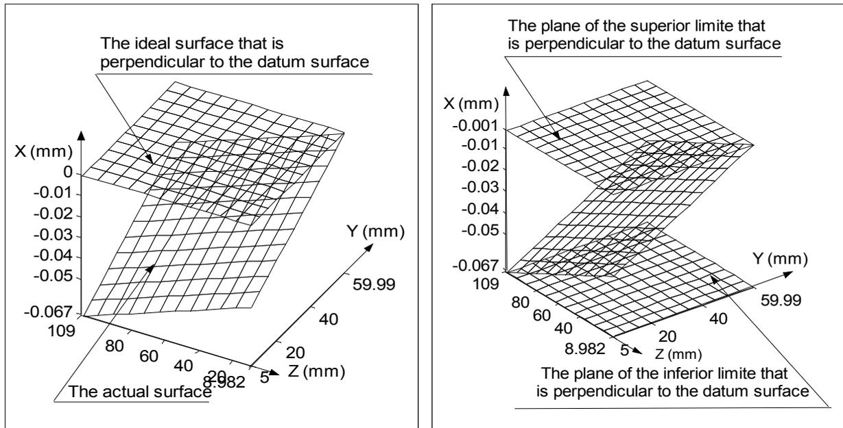
Figure 9: Geometric defaults that influence the perpendicularity of the machined surface 8 by report to the datum surface 9 while using the 1<sup>st</sup> fixture location
