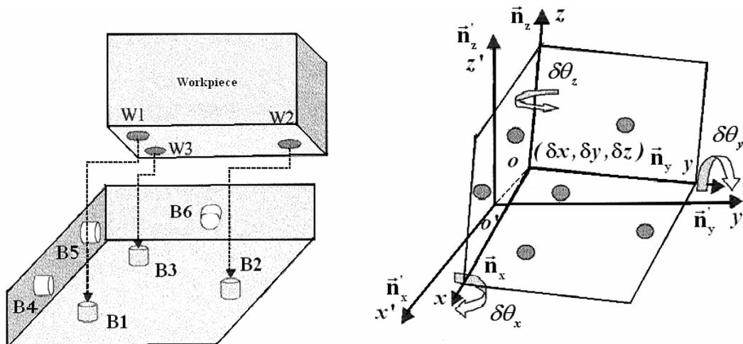
Figure 1: A 3-2-1 fixturing scheme and the related geometric errors ([12]).
