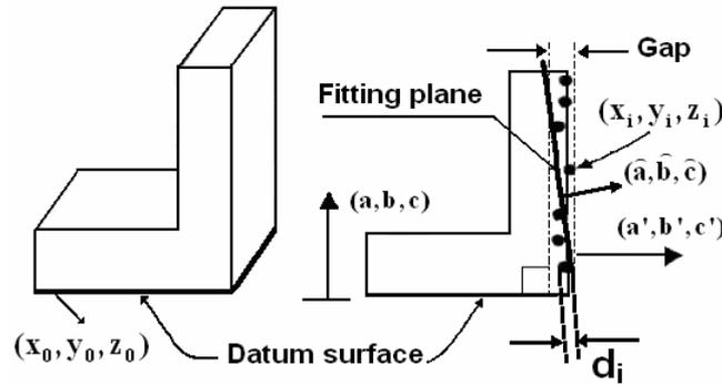
Figure 5: Interpretation of geometric defaults that influences the respect of the condition of perpendicularity
