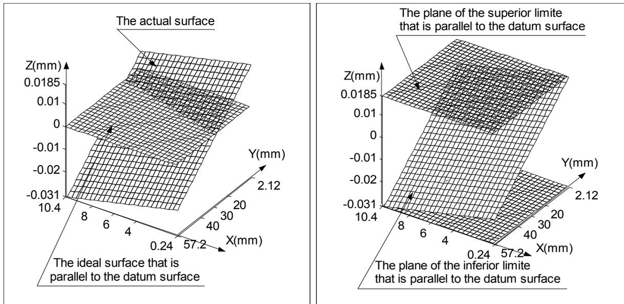
Figure 8: Geometric defaults that influence the parallelism of the machined surface 1 by report the datum surface 6 while using the 2<sup>th</sup> fixture location
