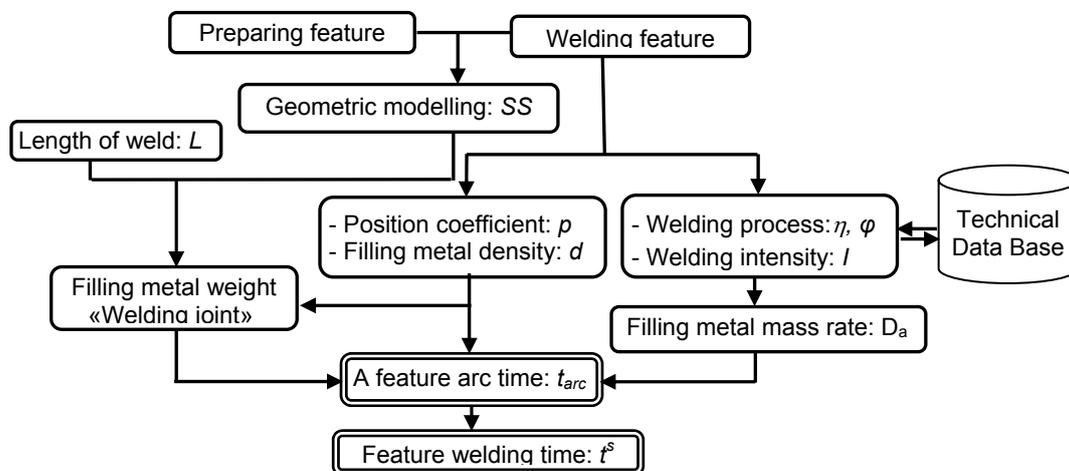
Figure 5: Welding time calculating methodology.
