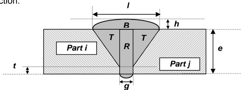
Figure 4: Geometric modelling of a welding feature "End to End" in V.
