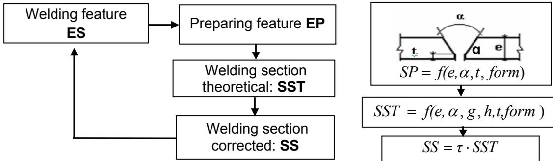
Figure 3: The geometric modelling approach of a welding section.
