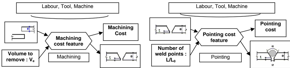
(a) The structure of the machining cost feature
