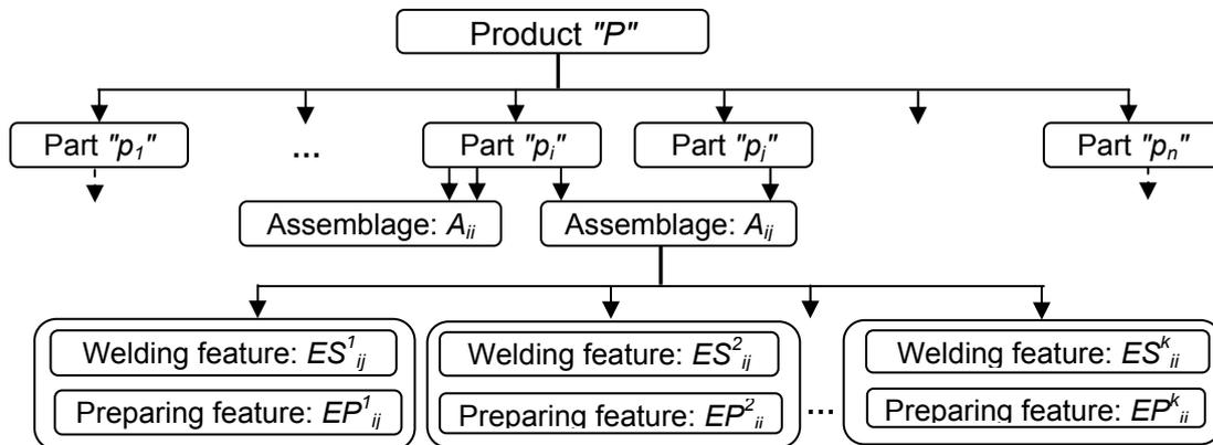
Figure 2: Approach for decomposition of "welding features" and "preparing features"
