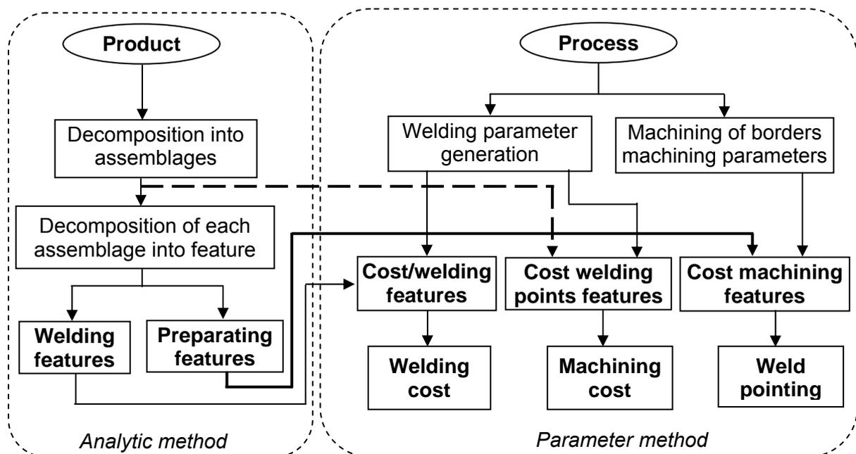
Figure 1: Model proposed for the welding cost estimation.
