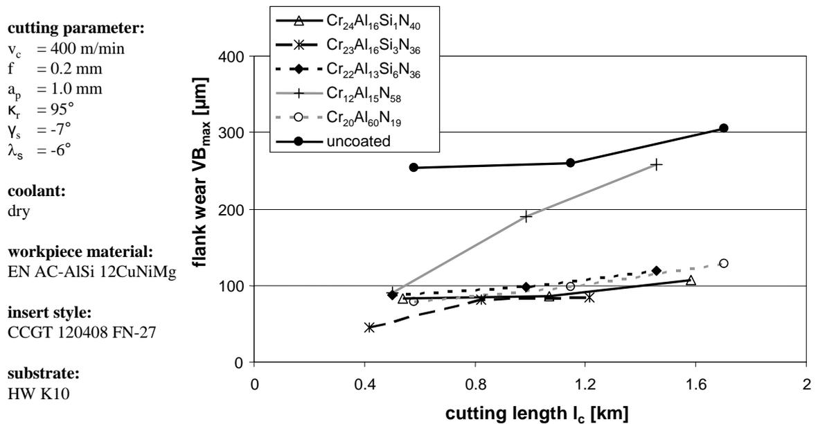
Figure 4: Development of flank wear versus cutting length for WC/Co coated tools in dry machining of an aluminium alloy.
