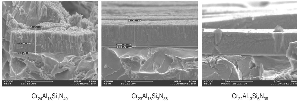
Figure 1: SEM pictures of fracture surface of CrAlSiN coated CK45 specimens.
