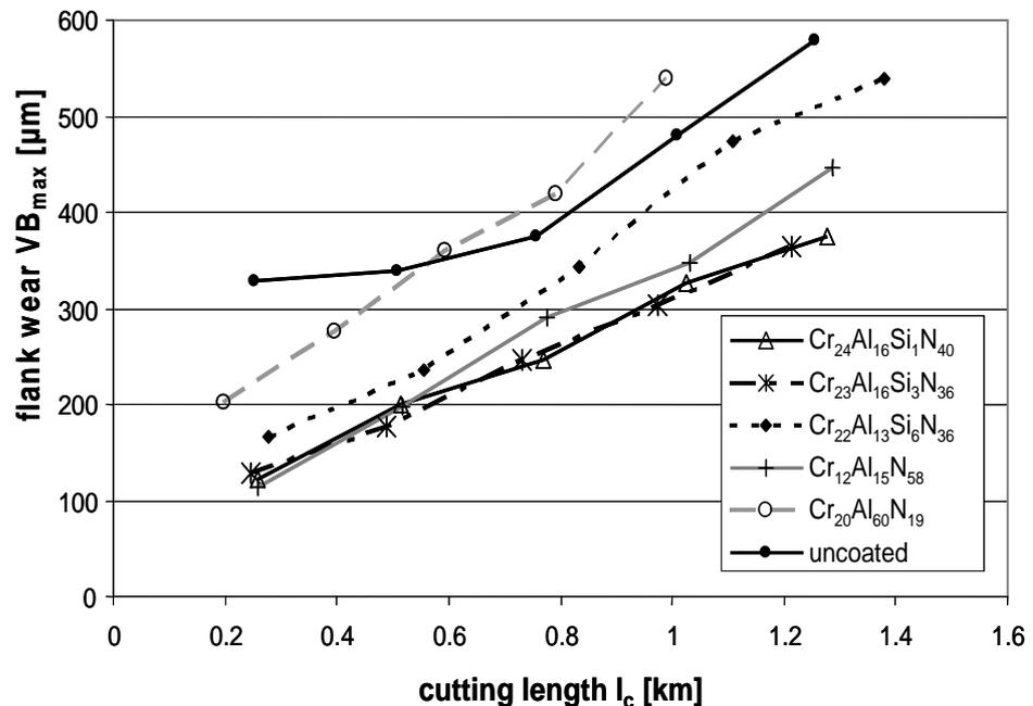
Figure 2: Development of flank wear versus cutting length for WC/Co coated tools in dry machining of spheroidal cast iron.
