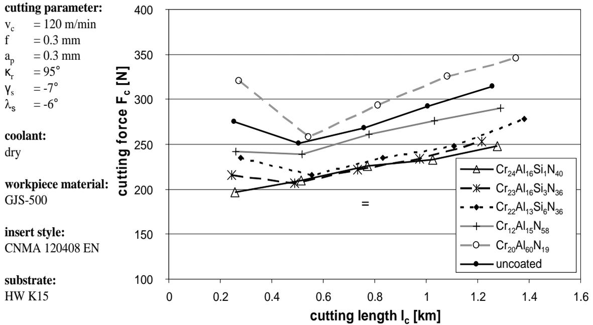
Figure 3: Development of cutting force versus cutting length for WC/Co coated tools in dry machining of spheroidal cast iron.
