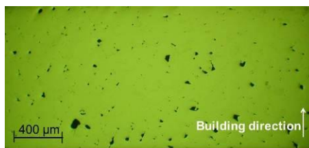
Figure 3: Cross-section of an SLM part with no laser re-melting.
