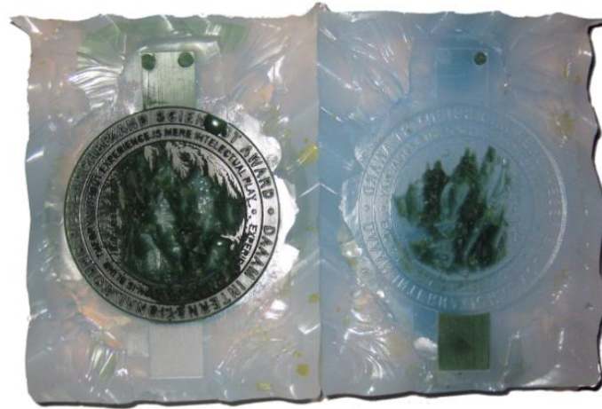
Figure 2: Damaged part as a result of still being in a liquefied state at the time of mould opening.
