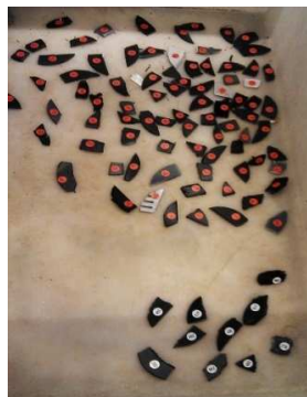
Fig. 3 Separation of black plastics labeled red (bromine) and white (no bromine) with XRT sensor based sorting
