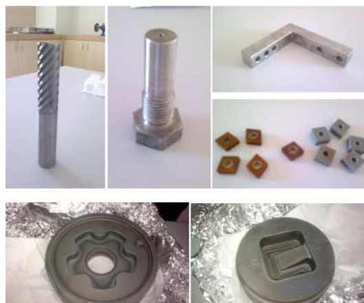
Fig. 3 Samples of coated parts-cutting tools & dies
