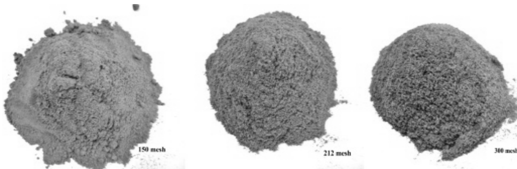
Fig. 1 Teak wood dust of three sizes: 150 \mu\text{m} (left), 212 \mu\text{m} (center), and 300 \mu\text{m} (right)
