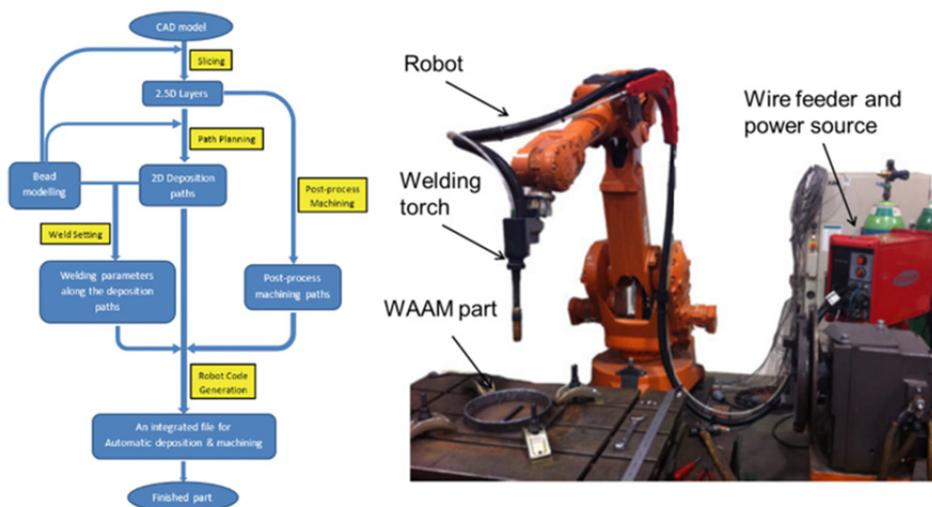
**Fig. 1** Scheme of WAAM process (left) and example of WAAM system (right) [8, 9]
