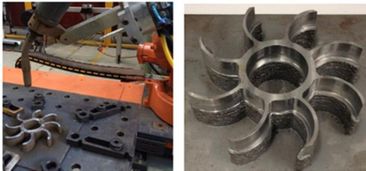
Fig. 2 Producing WAAM part (left) and partially post-processed part (right) [6]
