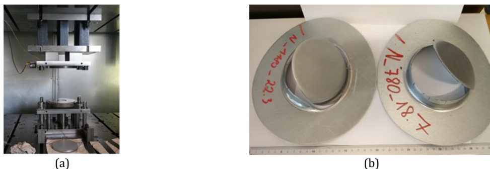
Fig. 1 (a) Experimental tool for deep drawing, (b) deep drawn cups ( v = 125 \text{ mm/s} , F_b = 200 \text{ kN} )
