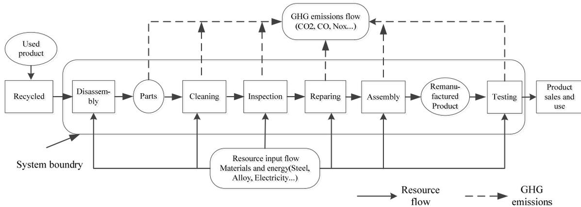
Fig. 1 GHG emissions boundary of mechanical product remanufacturing
