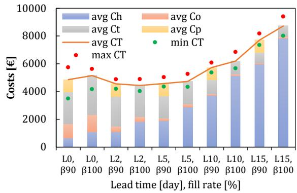
**Fig. 5** Minimum, maximum and average total costs and its components for  $\sigma_H$
