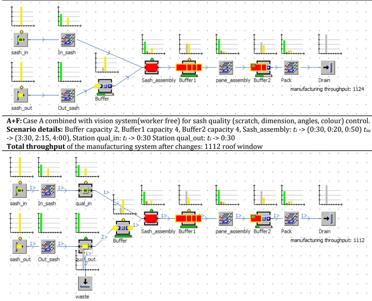
**A+F:** Case A combined with vision system(worker free) for sash quality (scratch, dimension, angles, colour) control.
