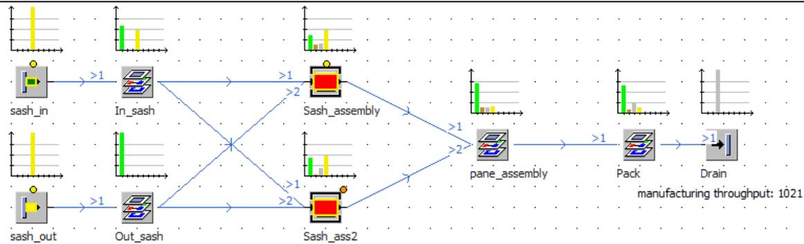
**A+C:** Case A combined with introducing the standardization on the station *sash\_assembly* for shortening processing and setup time.
