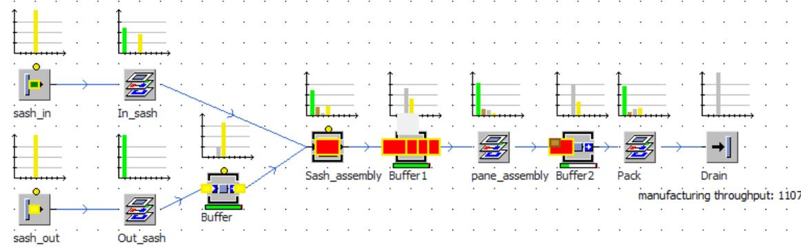
**A+D:** Case A combined with additional worker on *pane\_assembly*, who help in set-up. The scenario assumes panel computer installation, which shows setups ahead.
