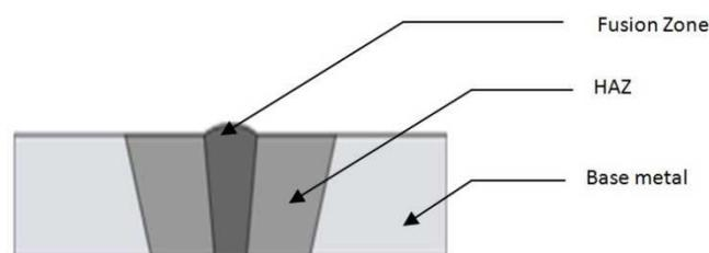
Fig 1: Cross-section of a butt weld joint
