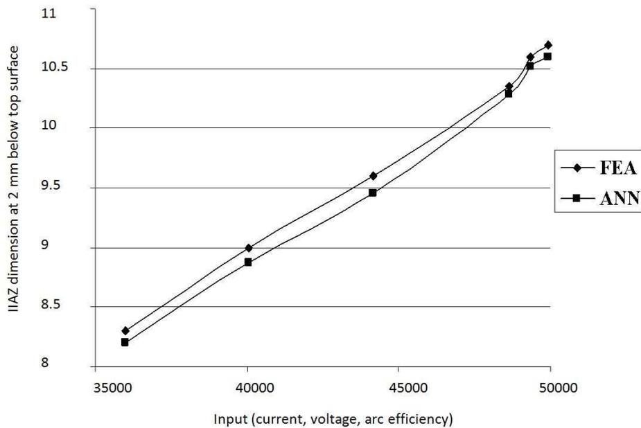
**Fig. 7** Comparisons of HAZ dimension at 2 mm below top surface of plate
