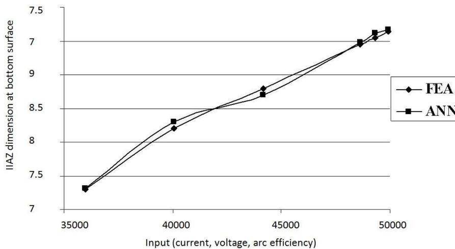
Fig. 9 Comparisons of HAZ dimension at bottom surface of plate
