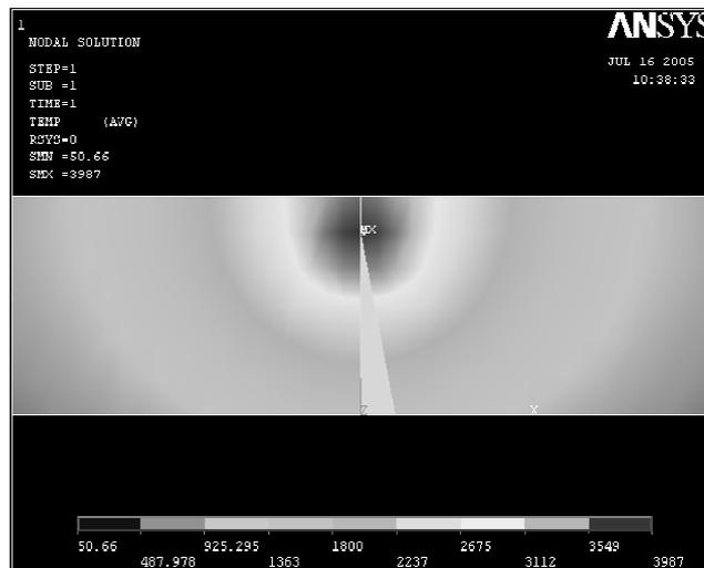
Fig. 3 Enlarged view of the HAZ
