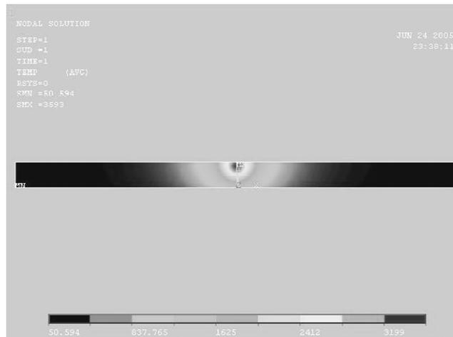
Fig. 2 Temperature distribution of welded plate
