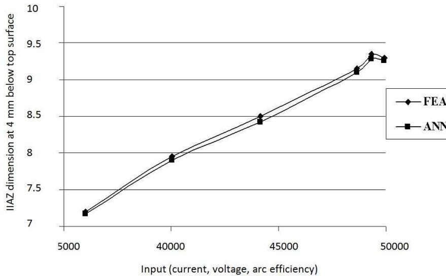
Fig. 8 Comparisons of HAZ dimension at 4 mm below top surface of plate
