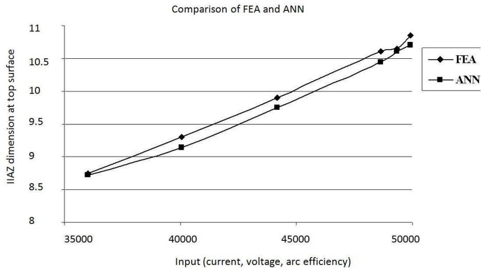
**Fig. 6** Comparisons of HAZ dimension at top surface of plate
