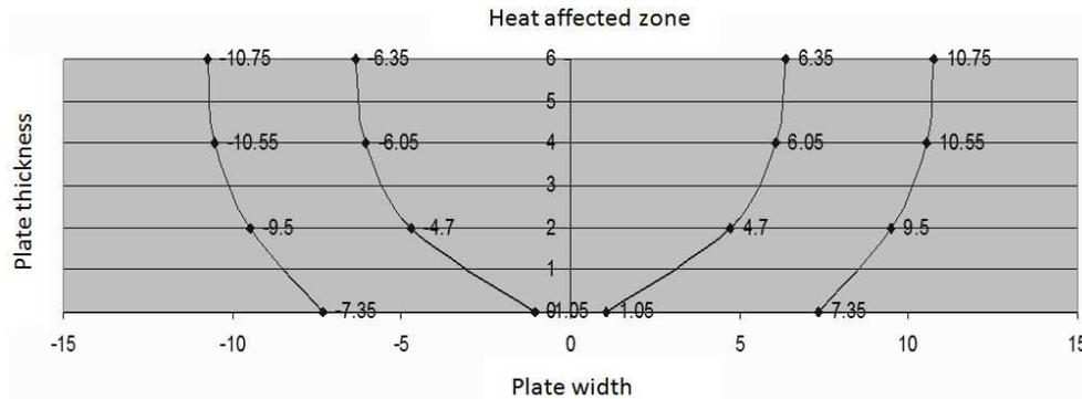
Fig. 4 Dimensions of HAZ
