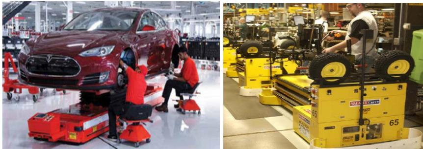
**Fig. 8** Service robots AGV applied in assembly process [28]
