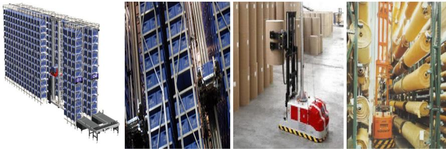
**Fig. 11** Service robots – AGV with telescopic forks
