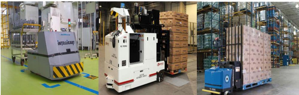
**Fig. 6** Service robots AGV trucks and pallet trucks [22,23]
