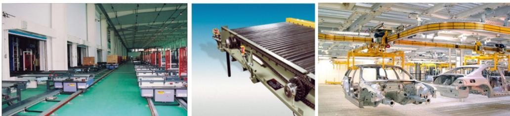
**Fig. 9** Rail guided vehicles, floor and overhead conveyors [28]
