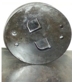
Fig. 10 Corner section die after assembly
