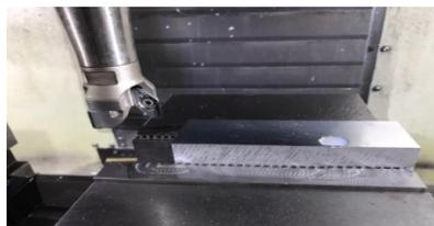
**Fig. 3** Experimental realization – clamping of the blank
