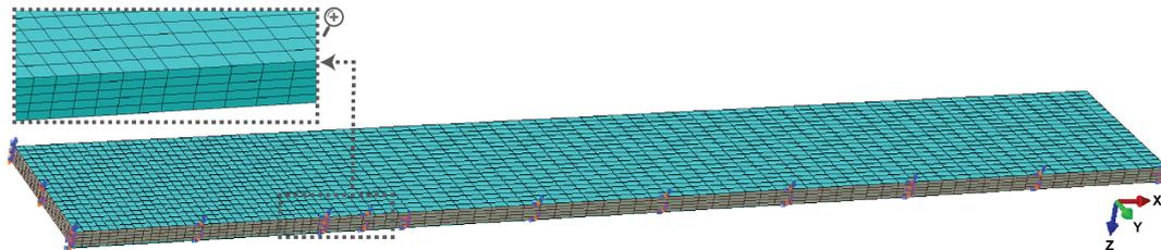
**Fig. 9** Symmetry boundary conditions and assigned mesh on the sheet metal for the three-point bending analysis
