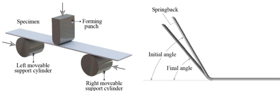
Fig. 8 Set-up of the three-point bending system and springback phenomenon
