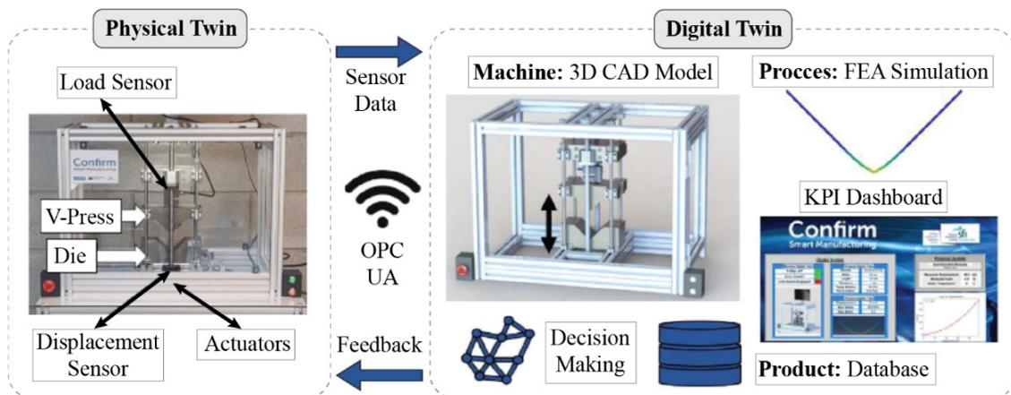
Fig. 6 Integration of physical and digital bending system [32]
