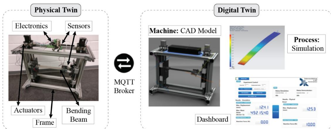
Fig. 7 Digital twin concept for bending beam test bench [34]
