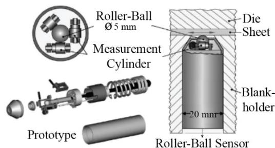
Fig. 3 Roller-ball sensor for material flow measurement [29]
