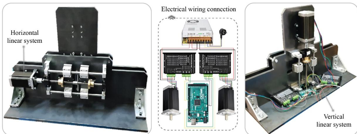
Fig. 17 Developed prototype of the flexible tooling system for sheet metal bending
