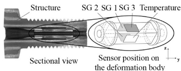
Fig. 5 Configuration of the sensor fastener [31]
