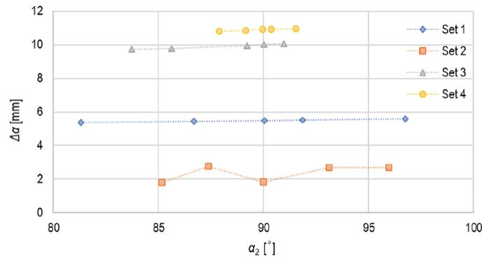
**Fig. 12** The relationship of the angle difference before and after springback,  $\Delta\alpha$ , and the bending angle after springback,  $\alpha_2$
