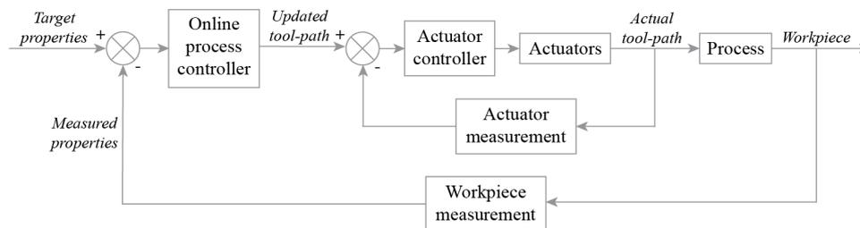
Fig. 1 A system diagram for closed-loop control of sheet metal forming process [15]
