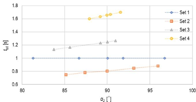
**Fig. 13** Total forming time,  $t_{tot}$ , required for obtaining different bending angles after springback,  $\alpha_2$
