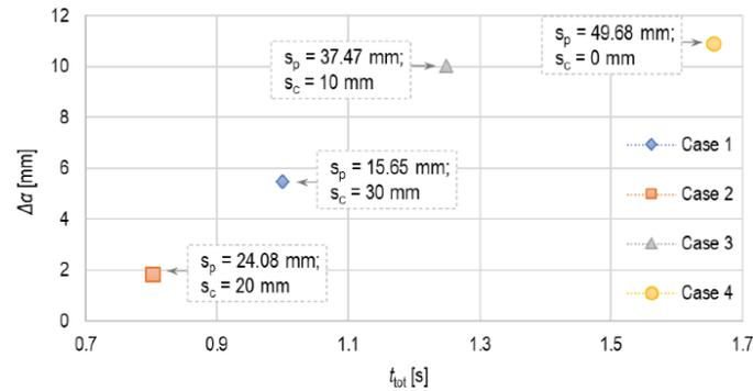
**Fig. 15** The relationship of the angle difference before and after springback,  $\Delta\alpha$ , and the total forming time,  $t_{tot}$ , when the bending angle after springback is  $90^\circ \pm 0.05^\circ$
