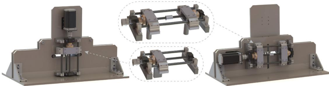
Fig. 10 3D model of the bending device with the vertical and horizontal linear systems
