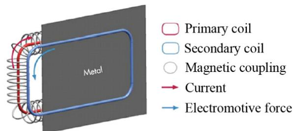
Fig. 4 Draw-in sensor based on the mutual inductance concept [30]
