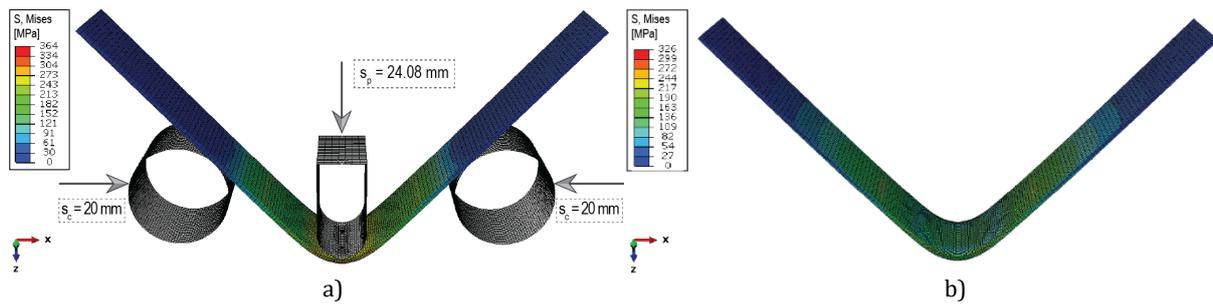
**Fig. 16** Visualization of the three-point bending model: a) loading step; b) unloading step
