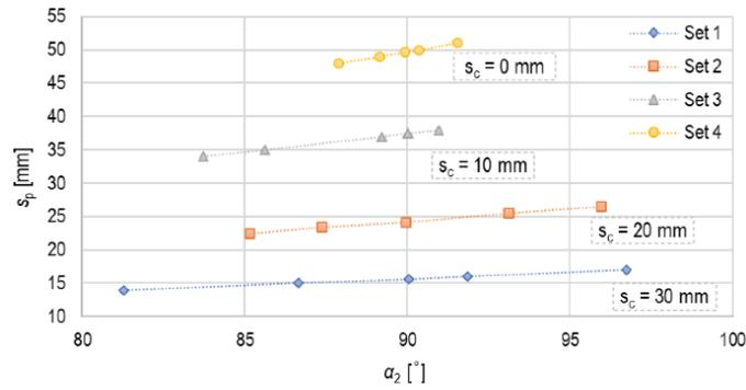
**Fig. 11** Displacement of the forming punch,  $s_p$ , versus bending angle after springback,  $\alpha_2$ , for different displacement of the support cylinders,  $s_c$
