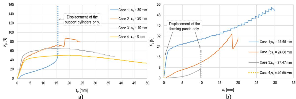
**Fig. 14** Forming force evolution in the cases in which the bending angle after springback is  $90^\circ \pm 0.05^\circ$ :
