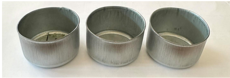
Fig. 9 Cups made of TRIP RAK40/70 steel after deep drawing test
