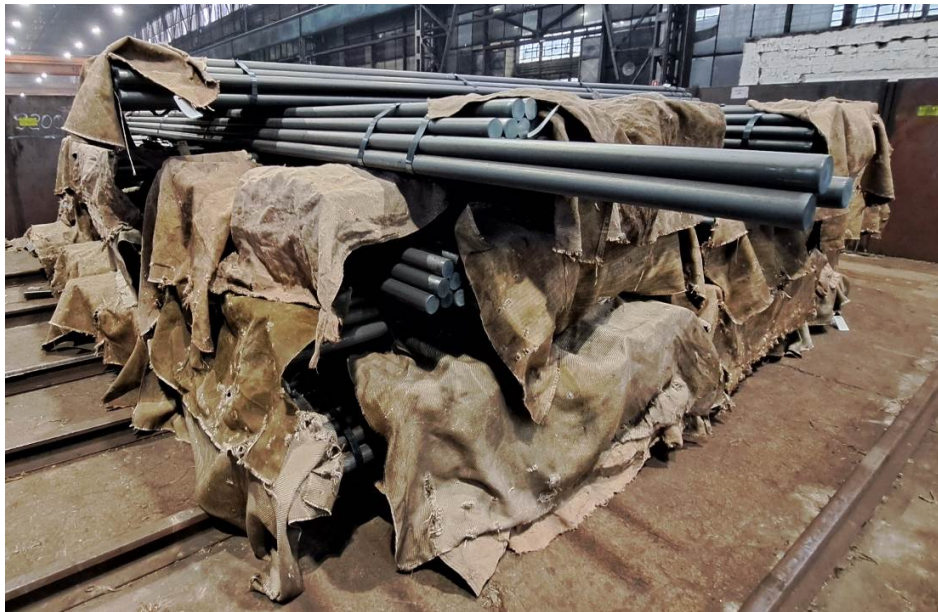
Fig. 1 The rolled round bars with insulation material (cloths) in the cooling chamber
