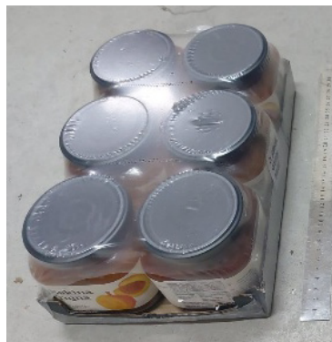
Fig. 3 Product for palletizing – package of jam jars with a mass of m = 6 kg
