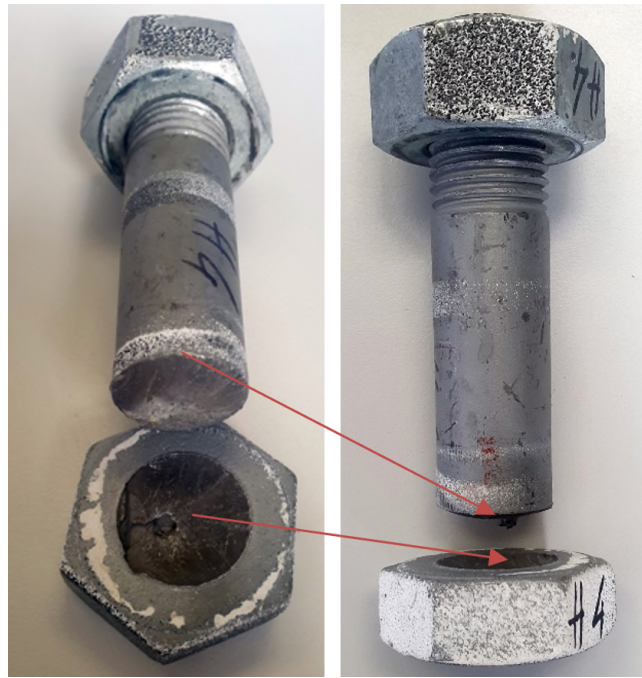
Fig. 2 Broken bolt that was received for testing
